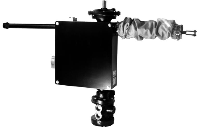
The major components for the direct-positioned pilot valve models include: a loading diaphragm assembly, pilot valve, the feedback return linkage, and a case containing the cam, pulley, levers, and linkages. When used on high-pressure hydraulic systems, where the pressures exceed 300 psig (21 kg/cm<sup>2</sup>), the pilot valve is operated by an auxiliary diaphragm.
