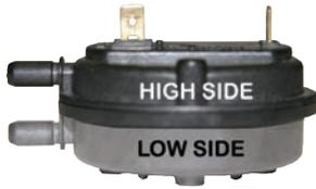
The entire field adjustable set point range of Series NS2™ switches is 0.10" w.c. to 10.0" wc, which is achieved by using five different range springs supplied along with the switch and other accessories in a contractor kit. When changing the set point of an air switch, do not exceed the maximum number of turns of the adjustment screw. For Series NS2™ switches, the maximum number of turns is given below for each of five standard set point ranges.
